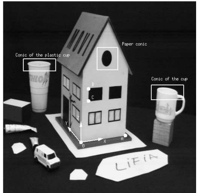
Fig. 3. One of the two original images in which the coordinate system for calibration and the conics used in the experimentation are marked. To have an idea of the real size of the object, OA and BC are measured as 13.75cm and 2.5cm .
