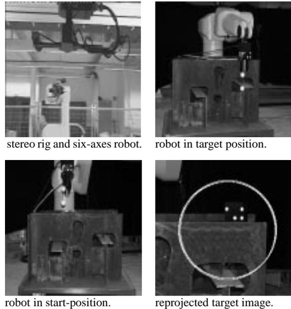
Figure 3: Overview of system for stereo visual servoing
