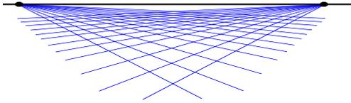
Figure 1: Vision geometry and its error model are essentially projective. Affine parametrization introduces an artificial singularity at projective infinity, which may cause numerical problems for distant features.
