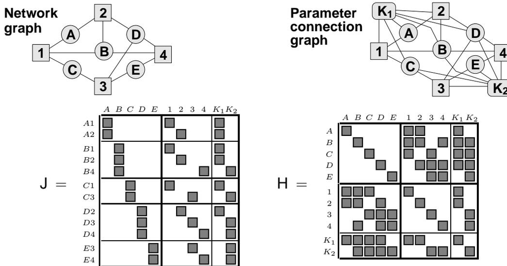
Figure 3: The network graph, parameter connection graph, Jacobian structure and Hessian structure for a toy bundle problem with five 3D features A–E, four images 1–4 and two camera calibrations  $K_1$  (shared by images 1,2) and  $K_2$  (shared by images 3,4). Feature A is seen in images 1,2; B in 1,2,4; C in 1,3; D in 2–4; and E in 3,4.
