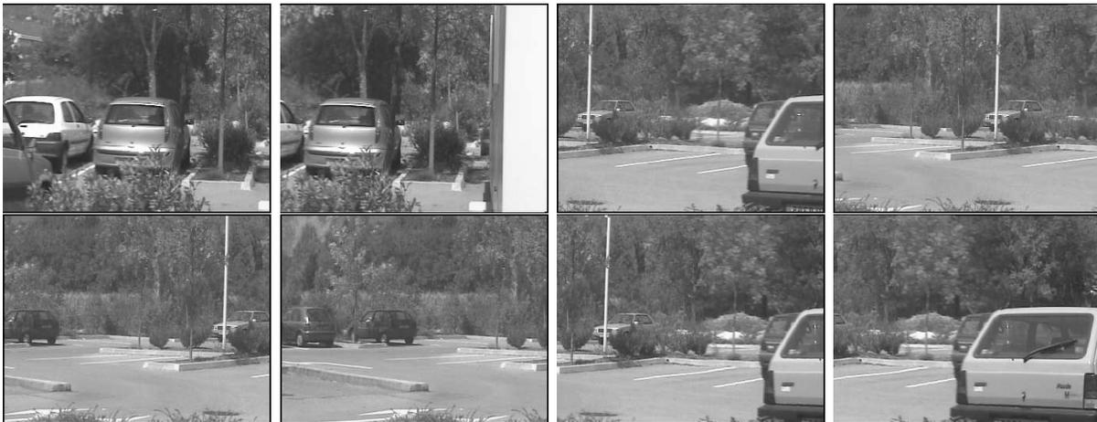
Figure 9: The foreground pixels were removed from the image sequence and replaced by background using the image-to-image homographies.
