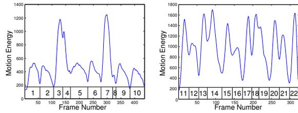
**Figure 3. Motion Energy for action: Lift arms - rotate arms - lower arms and turn in new position. Executed three times by (left) female actor, (right) male actor. Local energy minima serve as segmentation criteria of sequences. Motion volumes for each segment are shown in Figure 4.**
