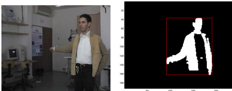
Fig. 1. Left. Training image of a person moving his right arm. Right. Feature extraction process: the object of interest is color segmented, and the bounding box (in red) around it is detected.
