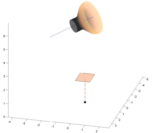
Figure 9. The calibration result showing the reconstructed mirror surface and its relative position w.r.t. the camera. The recovered angle is  $\alpha = 31.67^\circ$ .
