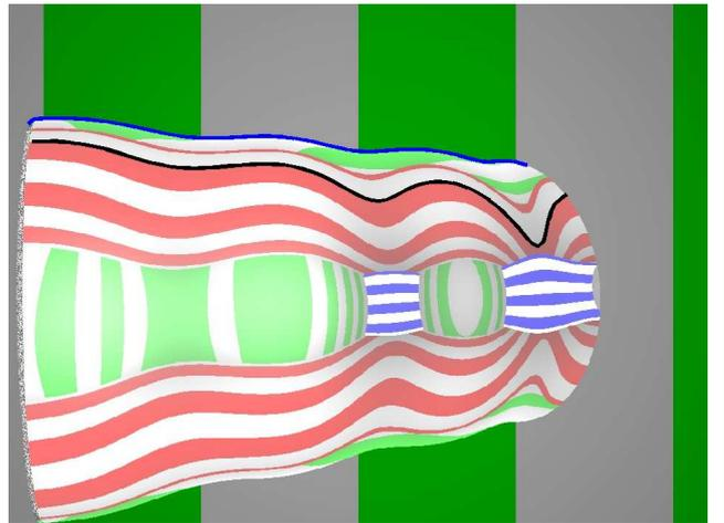
Figure 4. A second synthetic image showing the mirror, the extracted profile, represented in blue, and the used line image, shown in black. Also in this case the image of the visible cross section was not exploited
