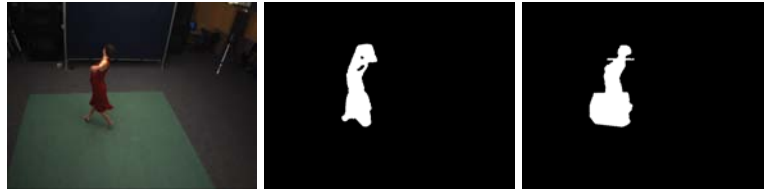
Fig. 3. Interim segmentation results with and without the spatial consistency. One of the input images(left) Segmentation result with the color difference only (middle) Segmentation result with the color difference and the spatial consistency(right)
