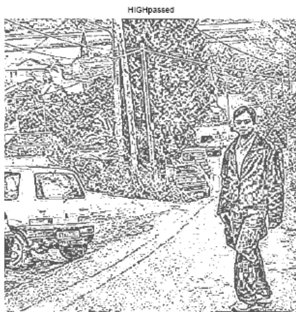
Fig. 16. Image passed through a 10 th order highpass filter with value of \alpha = 1.3 , sidebands 40dB down.
