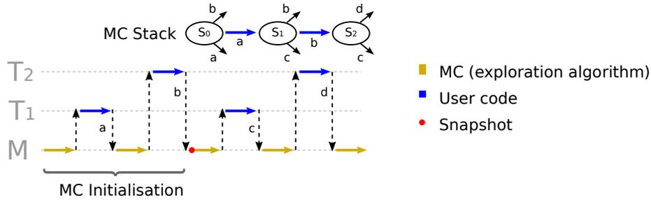
**Fig. 3.** State Exploration by SimGrid MC.
