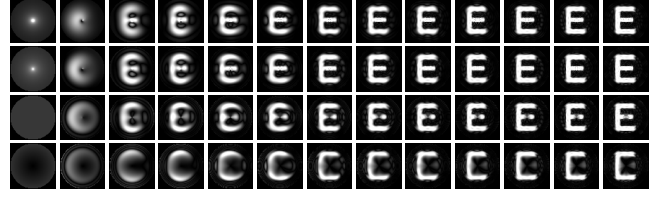
Fig. 4. Examples of reconstructed images of GPCET with s = 0.5, 1, 2, 4 (top to bottom rows) and L = 0, \dots, 12 .
