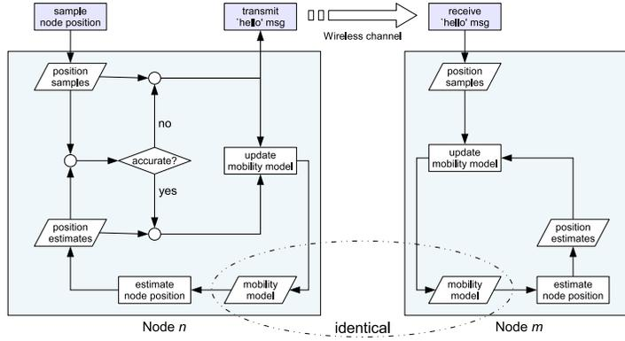
**Fig. 1.** Flow chart of ARH execution. Node  $n$  transmits ‘hello’ message according to the accuracy of its location estimates produced by an AR-based mobility model; node  $m$  is neighboring  $n$  and maintains an identical mobility model for  $n$ .
