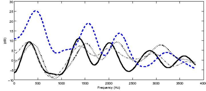
**Figure 3.** Natural and synthetic cepstrally smoothed spectra: dashed blue line (natural speech), black solid line (synthetic spectrum), gray dashed line (all coefficients adapted), dark gray dotted line (first two coefficients adapted only).
