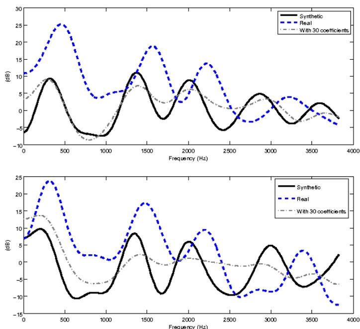
**Figure 2.** Natural and synthetic cepstrally smoothed spectra: dashed blue line (natural speech), black solid line (synthetic spectrum), gray dashed line (real spectrum adapted to fit the synthetic spectrum). All spectra are calculated with 30 cepstral coefficients.
