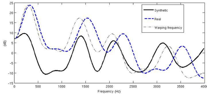
**Figure 4.** Natural and synthetic cepstrally smoothed spectra: dashed blue line (natural speech), black solid line (synthetic spectrum), gray dashed line (real spectrum after bilinear frequency warping).
