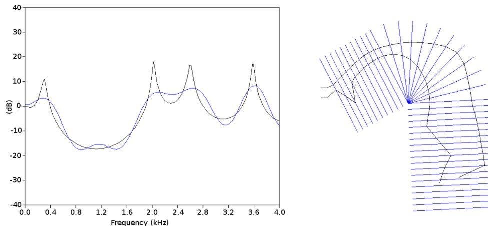
**Figure 1.** Simplified articulatory model and resulting synthetic spectrum. The spectrum with sharp peaks is the frequency simulation and the smooth curve is the cepstrally smoothed spectrum with 30 cepstral coefficients.
