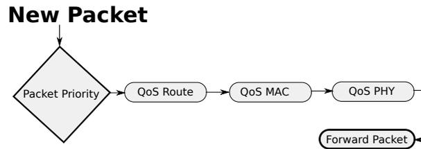
**Fig. 7.** Flow diagram at a Mobile Substitution Router.
