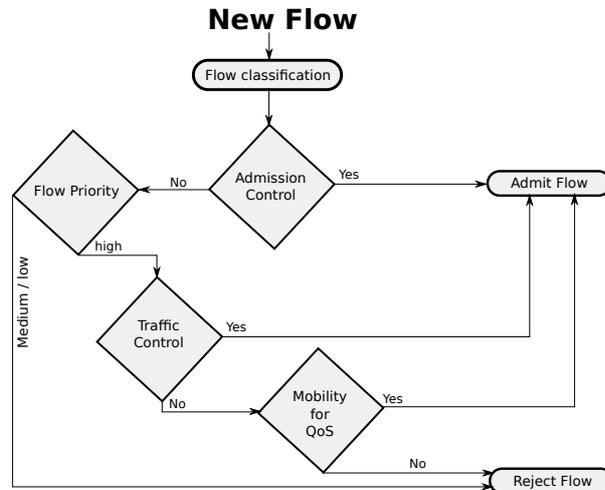
**Fig. 6.** Flow diagram at a Bridge Router source.
