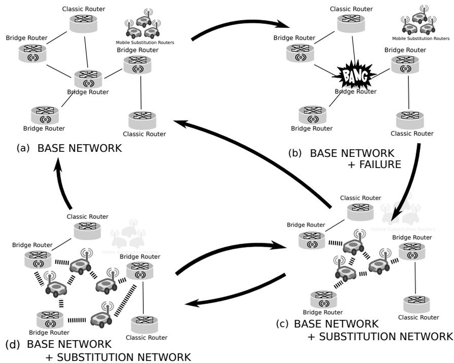
**Fig. 3.** Typical use case for a base network and a substitution network. Bridge Routers are deployed together with the base network. In case of failure, the mobile substitution routers are deployed or self-deployed to form a substitution network that helps the base network in restoring basic services such as connectivity.
