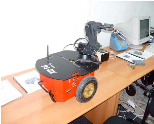
Fig.1: Mobile platform Pioneer 3-DX WMR.
