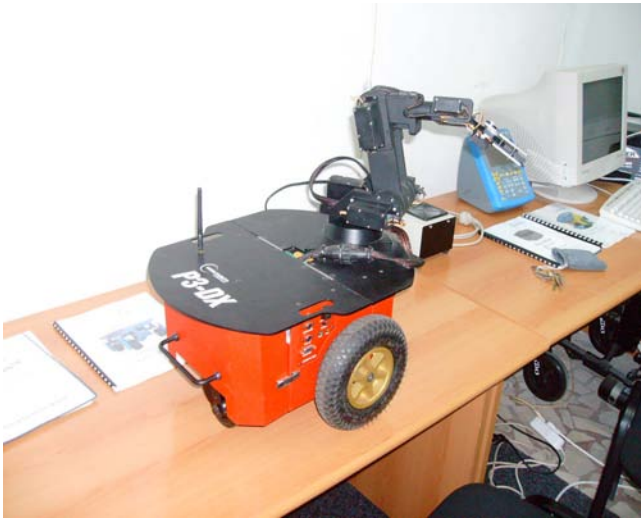
Fig.1: Mobile platform Pioneer 3-DX WMR.
