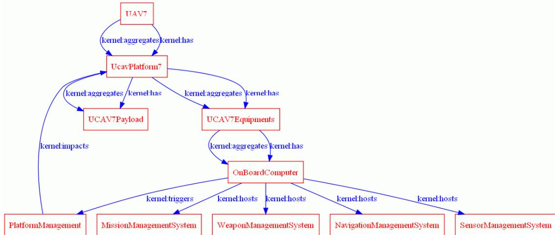
Figure 20: Software hosted in computer of UAV7
