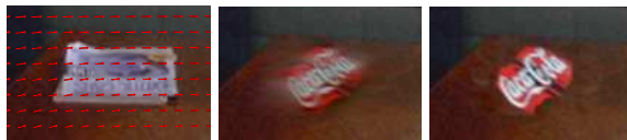
Fig. 1: Temporal consistency in gradient domain video editing. From left to right, a video frame with motion vectors superimposed, the result of video editing imposing the temporal consistency disregarding the motion of the scene, and the result of video editing considering the motion of the scene.
