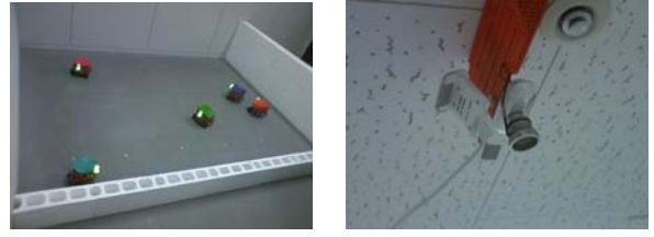
Fig. 3. Field (left) and the USB camera on the ceiling (right) of the environment of the experiments. For the field, the top leftmost corner is the origin; and x and y axes are along the thermocol blocks and the wall, respectively.
