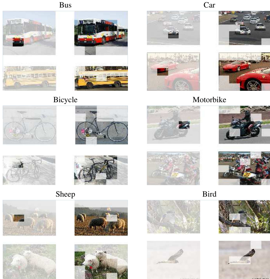
Figure 1: Examples of region classification by miSVM (left), and our RBLSTM (right). For visualization purposes, regions labeled as negative are marked by a transparent white mask.
