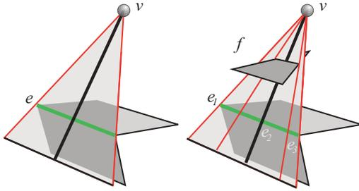
Figure 9: Swath validation. (a) The swath  $e_v$  is valid since the midline does not touch any other object. (b) The swath  $e_2v$  is invalid, since the midline is blocked by the face  $f$ , and the receiver has not been encountered.
