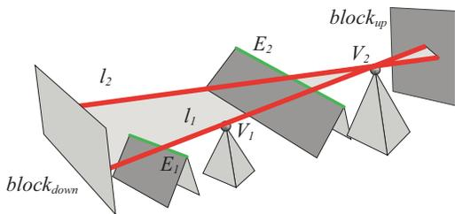
Figure 3: An extremal stabbing line  $l_1$ , with generators  $V_1, V_2, E_1, E_2$ , and up and down blockers  $block_{up}$  and  $block_{down}$ , and a swath between ESL  $l_1$  and ESL  $l_2$ , sharing  $E_2$  and  $V_2$ .
