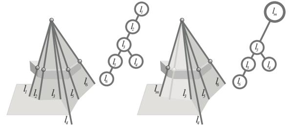
Figure 11: (Left) Original configuration with a small  $\epsilon$ . The corresponding graph is shown in the upper left. (Right) The  $\epsilon$  threshold is higher, and thus  $l_1$  and  $l_2$  will merge. A merged node  $l_m$  now takes the place of  $l_1$  and  $l_2$  in the graph.
