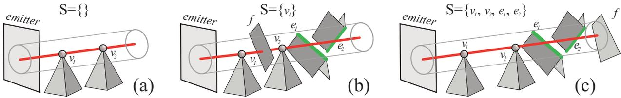
Figure 7: The ESL casting process. (a) Before casting, the line is formed by the native generators  $v_1$  and  $v_2$ ,  $S$  is empty and the line originates at the emitter. (b) The ESL encounters the generator  $v_1$ , and in this configuration, the ESL is invalidated by the face  $f$ . (c) Here, the ESL encounters generators  $v_1, v_2, e_1, e_2$ . This is a valid ESL, with down blocker  $f$ , since  $S$  contains the native generators.
