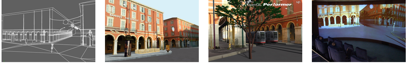
Figure 1. (left to right): wireframe of the 3D model reconstructed from a series of photos; the textured version of the model; the VE after the addition of virtual elements, shadows and lighting; the VE of the urban planning application as displayed on an immersive curved-screen display.
