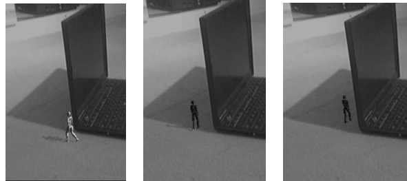
Figure 8: Results of the algorithm for an animated virtual avatar walking around a real laptop. Shadows are automatically detected and generated using our real-time algorithm.
