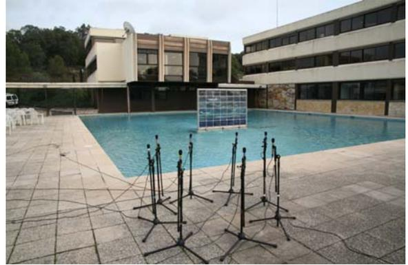
Figure 14: Microphone setup used to record the fountain example. In this case the microphones are placed at the center of the action.
