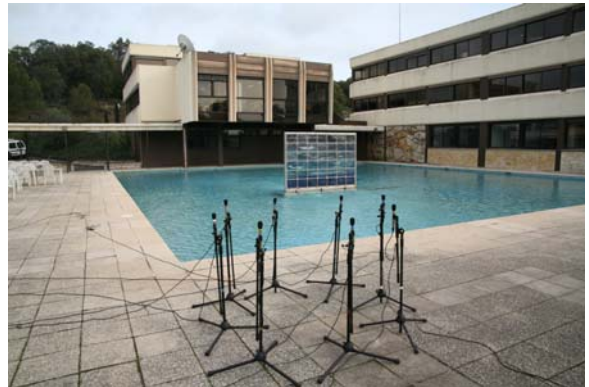
Figure 14: Microphone setup used to record the fountain example. In this case the microphones are placed at the center of the action.
