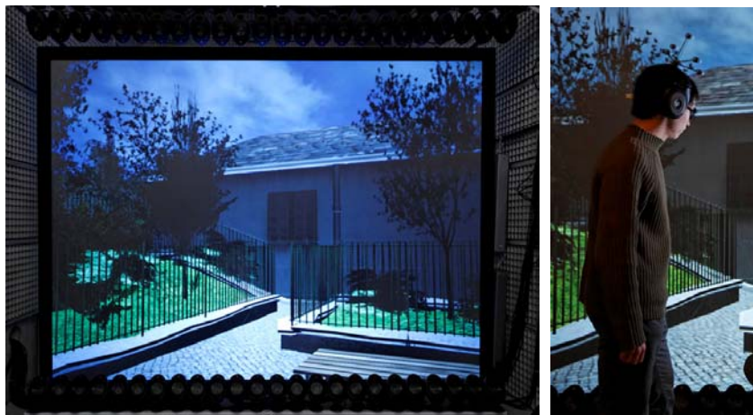
Figure 2. Virtual Reality setup. On the left, view of the entire screen in the acoustically damped studio, on the right, a participants equipped with headphones, a head tracker and polarized glasses.
