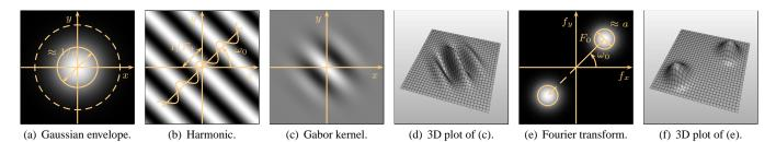
Figure 2: The Gabor kernel. (a) Gaussian envelope. (b) Harmonic. (c) Gabor kernel. (d) Gabor kernel, 3D plot. (e) Fourier transform of Gabor kernel, 3D plot.
