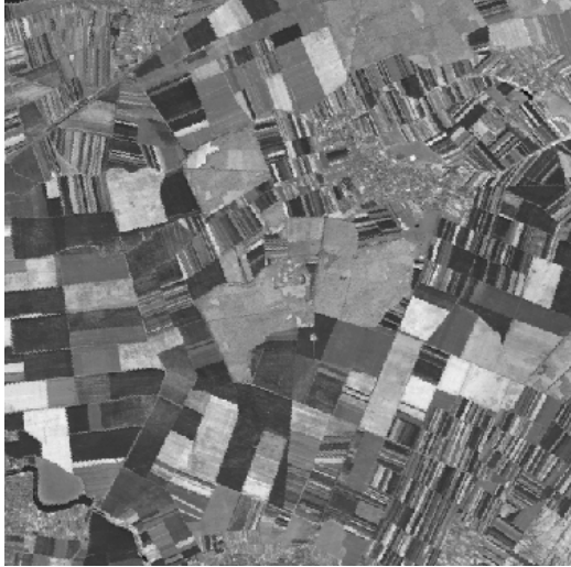
Figure 1: High-resolution Spot image ( 20 \times 20 m per pixel) acquired in the Near Infrared channel. In this scene, we can recognize some fields, roads and also poorly delimited areas which correspond to cities.
