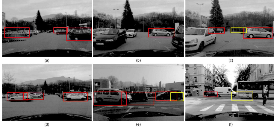
Figure 6: Car-side detection examples. True and false positive detections are represented by red and yellow bounding boxes respectively. (a) Cars in different scales with significant background clutter and significant occlusions are detected. (b) Precise detection of the un-occluded vehicle, whereas a vehicle that is heavily occluded in the left is not detected. (c) Difficult detection of a vehicle which is far and partially occluded and a false detection in the region between the road surface and the trees. (d) Detection with partial occlusion. (e) Partial detection of a taller than normal vehicle (on the left). The training dataset does not contain vehicles of this type. (f) Successful detection of a partially occluded car and a false positive arising from a bus and a van. Training separate detectors for these type of vehicles as well will help to avoid these false alarms.
