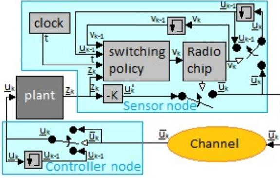
Fig. 1. Block diagram of the problem setup. The sensor node measures the state  $z_t$  from the plant and decides whether to send it or not to the controller node.  $\bar{z}_t$  is equal to  $z_t$  when a transmission occurs, or to  $\emptyset$  otherwise. The controller is then able to determine if a transmission has occurred or not.
