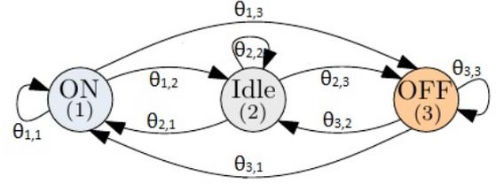
Fig. 2. Illustration of the transitions costs. Idle represents an intermediate mode between ON and OFF. The  $\theta_{i,j}$  represent the energy costs associated to the transition from mode  $i$  to mode  $j$  and  $\theta_{i,i}$  the cost to stay in mode  $i$ .
