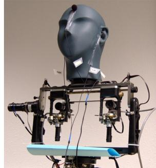
**Figure 1:** The POPEYE robot head is the audio-visual recording device used to acquire the Ravel data set. The color camera pair as well as two (front and left) out of four microphones are shown in the image. Four motors provide for the rotational degrees of freedom and ensure the stability of the device and the repeatability of the recordings.
