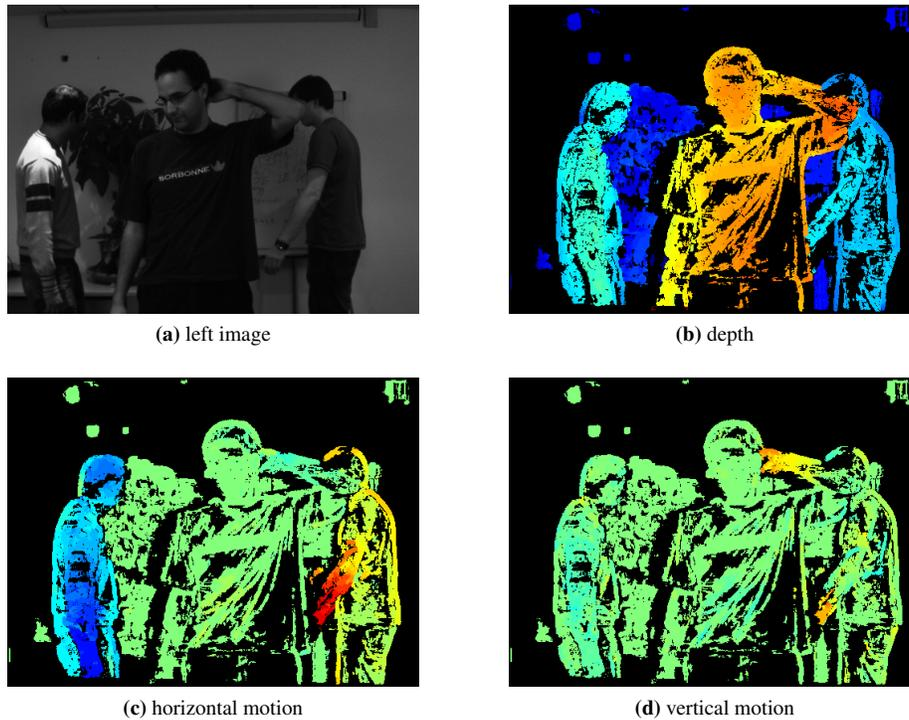
**Figure 4:** Scene Flow. The results are color coded. For disparity map (b), warmer colors are closer to the camera. For optical flow maps (c) and (d), green color stands for zero motion, while colder colors correspond to right and up motion respectively, warmer colors the opposite direction. Black color stands for unassigned disparity or optical flow.
