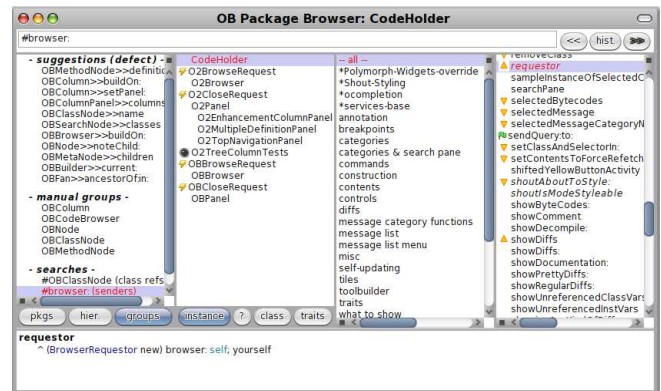
Figure 2. SmartGroups view integrated on the left side of Pharo Smalltalk’s system browser, the core of the Smalltalk IDE.
