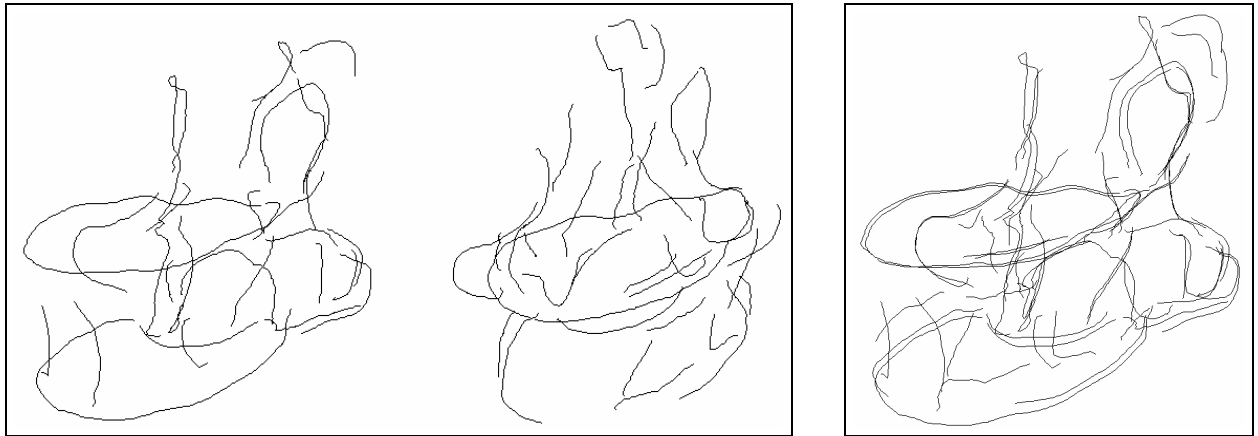
Figure 6: (a) Left: Crest lines on two 3D CT images of a vertebra. (b) Right: Superimposition of the lines of a. with our software in 8.9 seconds CPU on a DEC 5900. 12 curves were identified out of 28 and 33. 82 points were identified among these curves out of 1250 and 1213 points respectively in the two different sets of curves.
