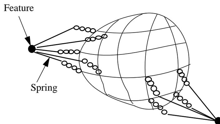
Figure 3 For every feature, we attach springs to all nodes of the surface
