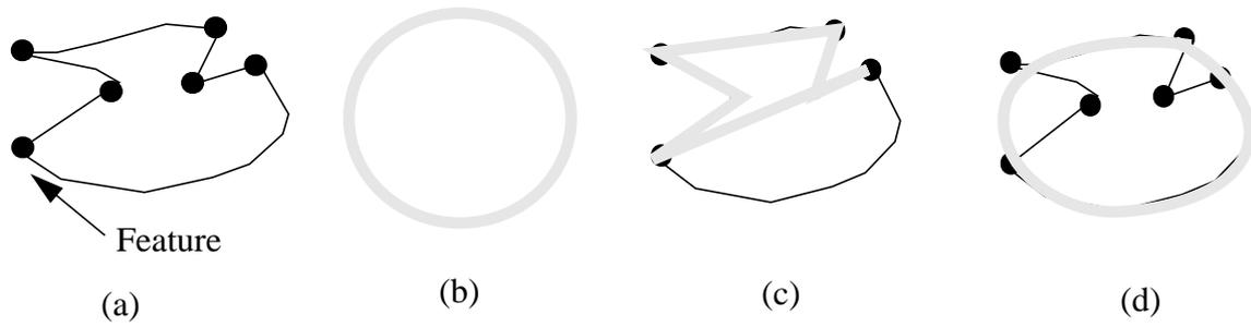
Figure 4 **a**, An object with its features (normal discontinuities); **b**, Surface initialization; **c**, Final shape if feature deformation is predominant; **d**, Final shape if data deformation is predominant
