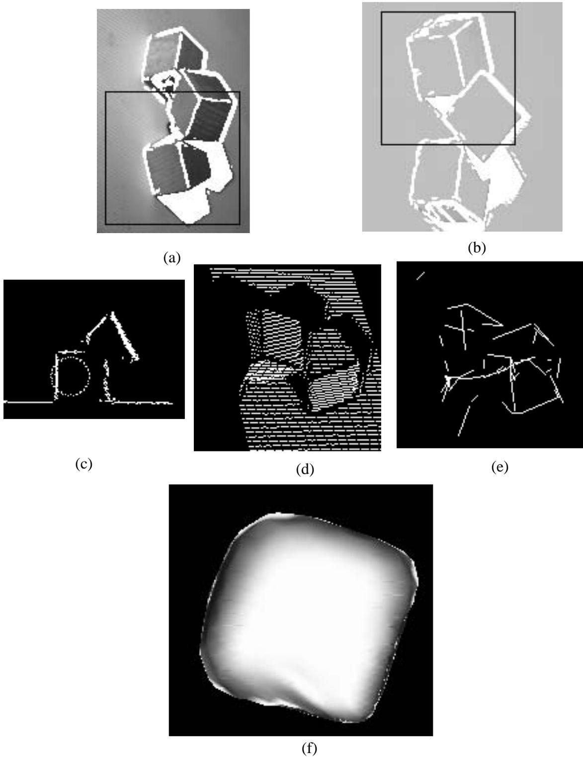
Figure 16 **a**, First range image with features; **b**, Second range image with features; **c**, **d**, and **e**, Initialization, range data and features for the extraction of the first cube; **f**, First cube reconstructed by the deformable surface;
