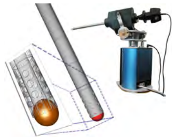
Figure 4: Picture of the ITP Xitact tool and its corresponding model. The tool tip corresponds to a sphere collision model.
