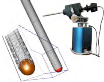
Figure 4: Picture of the ITP Xitact tool and its corresponding model. The tool tip corresponds to a sphere collision model.
