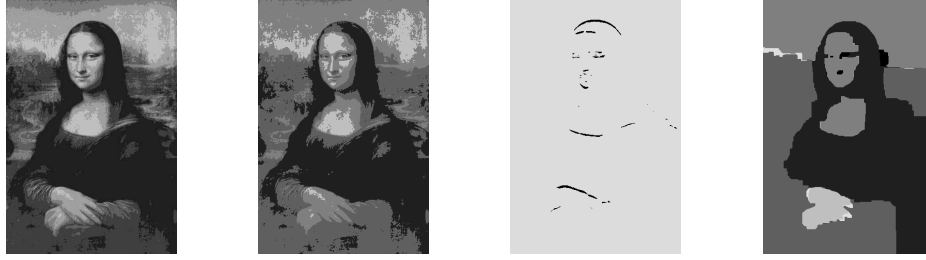
Figure 4. An example of image digitalization in 8 grey levels, with edges enforced, in the same spirit as in Figure 3. We consider 8 classes of grey levels. The individual potentials rely on the intensity of pixels. The coherency criterion makes use of an edge detector and enforces label variations on edges. From left to right : most probable grey level (at each pixel independently) of the original potentials; of the potentials once projected on the set of admissible potentials ( i.e. on \mathcal{F}_0 ); edges enforced; result. It is possible to let the user interact with the process and add edges manually to obtain new digitalization results. The interaction matrices used are (a) and (b) in Table 1.
