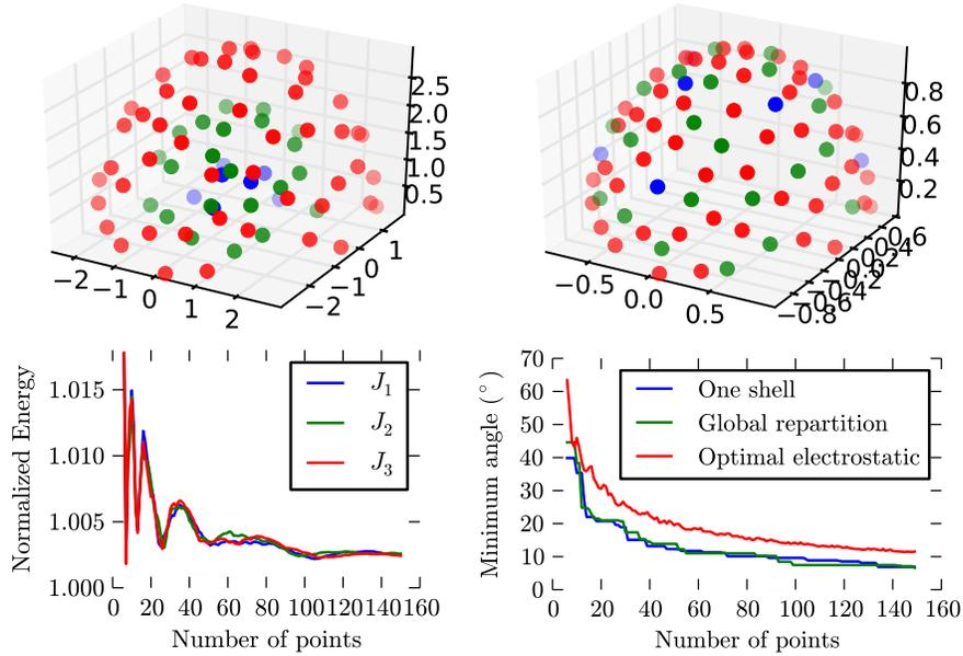
**Fig. 2.** (top left) Multiple  $q$ -shell experiment design: 120 points on 3 shells, with  $N(q) = q^2$ . (top right) Points reprojected on the unit sphere. The distribution of points on each shell is uniform, as well as the global angular density. (bottom left) Normalized electrostatic energy. (bottom right) Minimum angle between any two points.
