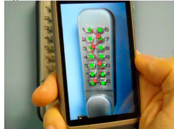
Figure 1. AR layer for passcode entry: the user “scans” a keypad with a camera phone; once the keypad is recognized, the phone displays animated tapping footprints between the keys to illustrate the required key sequence (passcode) for unlocking the door.
