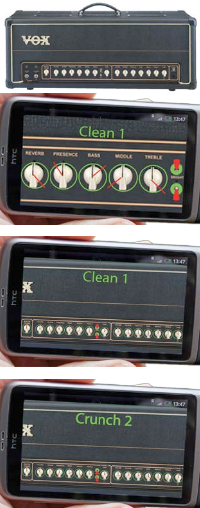
Figure 2. Displaying AR notes on a guitar amplifier for different settings with different zoom levels.
