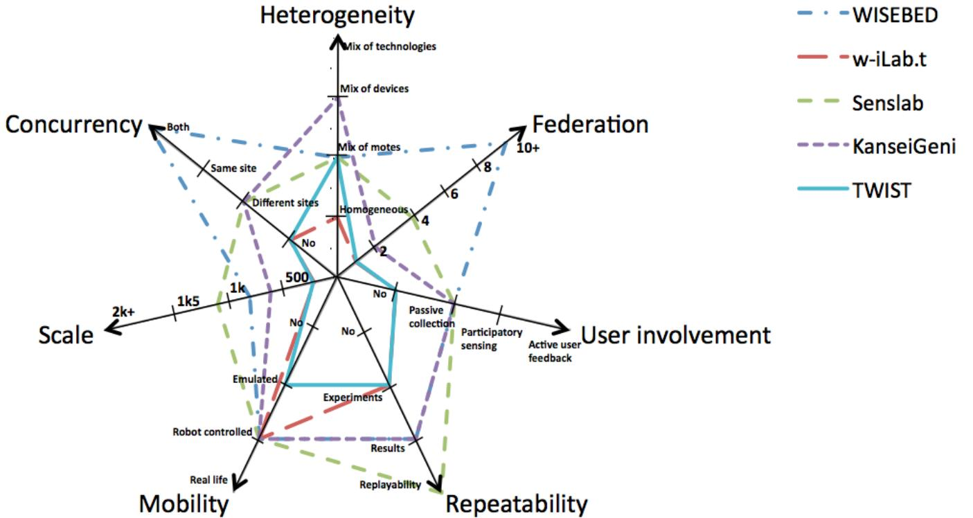
Fig. 5. Mapping of features of current testbeds to identified requirements.
