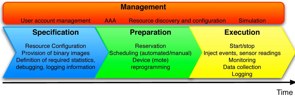
Fig. 4. Experiment execution workflow and corresponding testbed services.
