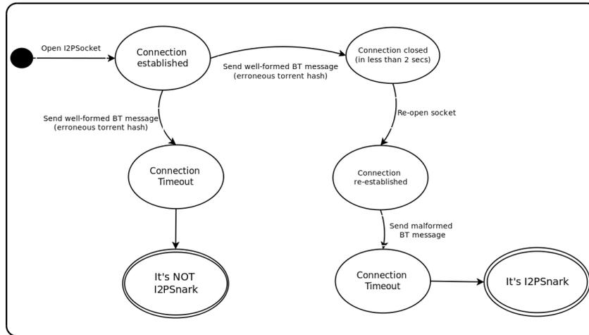
**Fig. 3.** State machine for testing an I2PSnark client
