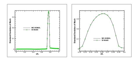
Figure 9: Nozzle flow with uncertain  $\gamma$  (discontinuous pdf) and  $p_e$  (uniform pdf). Standard deviation for the Mach number distribution for MC-SOBOL and SI methods. Left : global view; right : close-up on the shock region.
