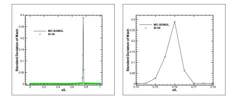
Figure 8: Nozzle flow with uncertain  $\gamma$  (discontinuous pdf). Standard deviation for the Mach number distribution for MC-SOBOL and SI methods. Left : global view; right : close-up on the shock region.
