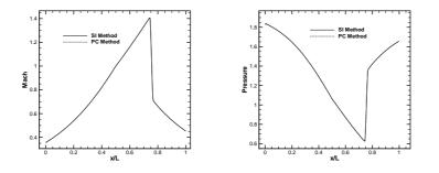
Figure 6: Nozzle flow with uncertain  $\gamma$  (uniform pdf). Computed mean distribution for the Mach number (left) and the static pressure (right) using the semi-intrusive method with 10 points in the probabilistic space and the PC method with a 10th order polynomial.
