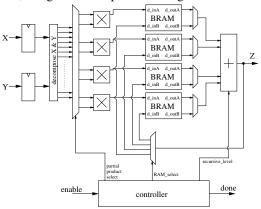
Figure 5. DSP48E and BRAM based Multiplier
