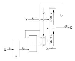
Figure 2. Serial Multiplier
