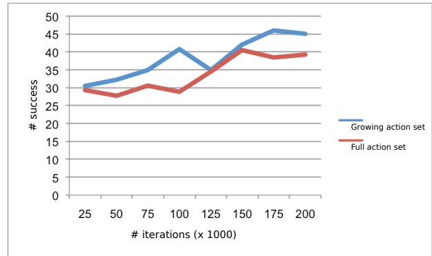
Fig. 5. Using configuration (1). Directly learning with the full set of actions is less efficient than learning with only 3 actions and, then (around iteration 100.000) using 5 actions. This results comes from only one experiment with the robot, as policy evaluation, done every 25.000 iteration, takes about 20 minutes.
