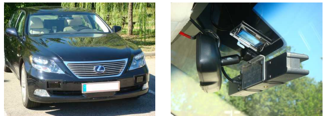
Fig. 2. Our experimental platform on a Lexus car, with a TYZX stereo camera behind the windshield and two IBEO Lux lidars inside the frontal bumper
