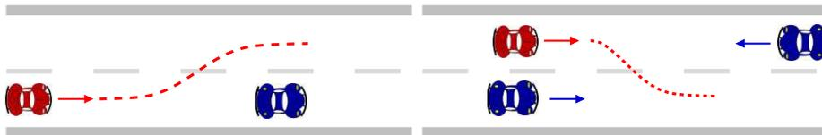
**Fig. 1.** Collision avoidance model scenarios: stationary obstacle (left) and overtaking maneuver (right)
