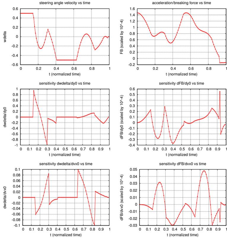
**Fig. 4.** Sensitivity differentials for the optimal controls of OCP( $\hat{y}_0, \hat{v}_{x,0}$ ) at  $\hat{y}_0 = 1.75$  and  $\hat{v}_{x,0} = 35$ : Control and sensitivities of  $w_\delta$  w.r.t.  $y_0$  and  $v_{x,0}$  (left) and of  $F_B$  w.r.t.  $y_0$  and  $v_{x,0}$  (right).
