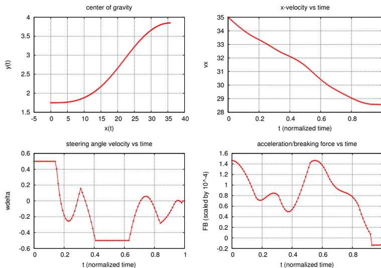
**Fig. 2.** Avoidance trajectory for  $v_{x,0} = 35$ ,  $y_0 = 1.75$ ,  $y_{target} = 3.85$ : center of gravity and velocity in x-direction (top), steering angle velocity and braking/acceleration force (bottom). The distance  $d$  computes to 35.6798 and the final time  $t_f$  to 1.1399.
