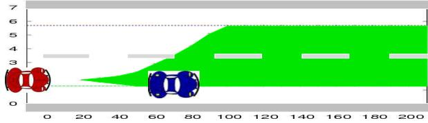
**Fig. 3.** Projected reachable sets for initial velocities  $v_{x,0} = 75, 100, 150, 250$  [km/h]. The approaching car can avoid a collision with the obstacle in the first three settings, but not in the final setting, if the measurements of the obstacle and the approaching car are taken into account.
