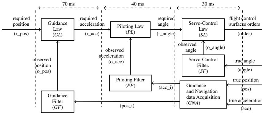
**Fig. 1** A simplified flight control system (FCS)
