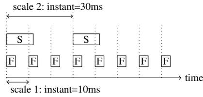
**Fig. 4** Logical time scales in a multi-periodic system
