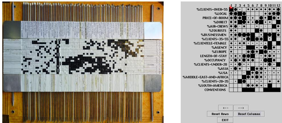
Figure 2.5: The reorderable matrix. On the left one of Bertin’s physical matrices; on the right an implementation of the reorderable matrix by drag and drop of rows and columns [Siirtola, 1999].
