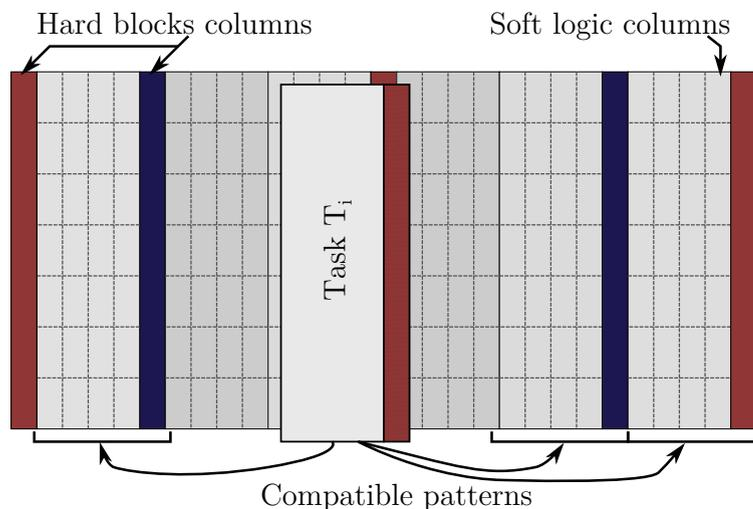
Figure 2-2 – Becker *et al.* [BLC07] solution to logic fabric heterogeneity. The solution brought by [BLC07] handles more compatible patterns on the logic fabric, but they are not usable by the tasks. Considering task  $T_i$ , any hard block can fit its hard block slot, as long as its relative position to the soft logic is kept.
