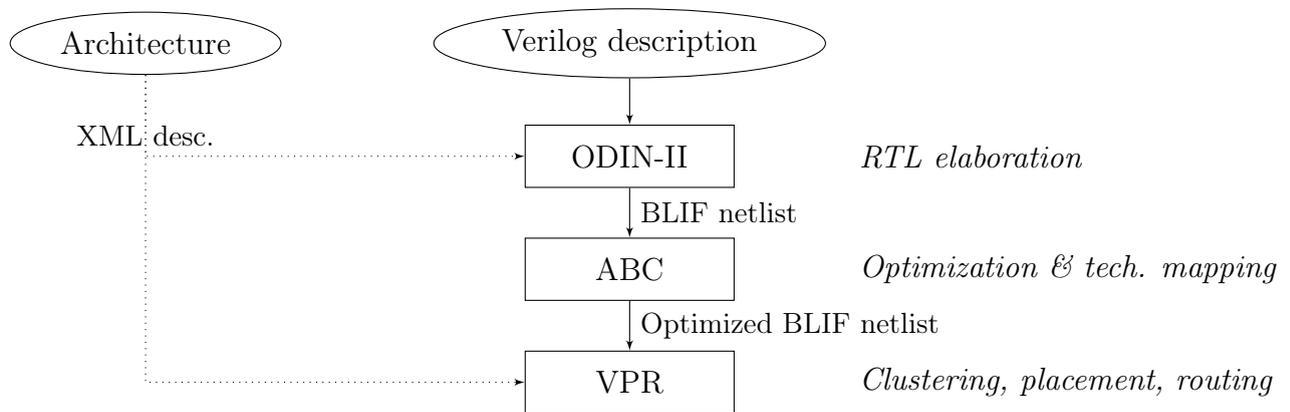
Figure 2-5 – The Verilog to Routing design flow
