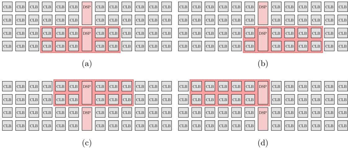
Figure 5-4 – **Multiple relocation possibilities for the same bit-stream of a task.** *As the connections between the homogeneous routing and the hard blocks can be made at multiple equivalent points of connection within switches, the task benefits from an increased flexibility in its horizontal placement. The vertical placement possibilities are still limited by the common denominator of the hard blocks heights.*
