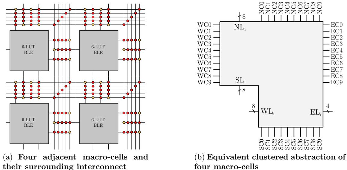
Figure 3-6 – **Clustering multiple macro-cells together before coding the Virtual Bit-Stream.** *Using the Virtual Bit-Stream technique, it is possible to use a coarser level of abstraction by grouping multiple macro-cells together prior to the calculation of the route list. The clustering offers the possibility to represent the routes with even fewer data, but at the cost of more complex decoding operations.*
