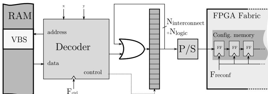
Figure 4-1 – **Architecture of the decoding part of the online controller.** The decoder (*de-virtualizer*) is responsible for the decoding of the macro-cell data contained in the Virtual Bit-Stream files. Each macro-cell is decoded to a full conventional bit-stream containing  $N_{interconnect}$  interconnect configuration bits and  $N_{logic}$  hard block or soft logic configuration bits.
