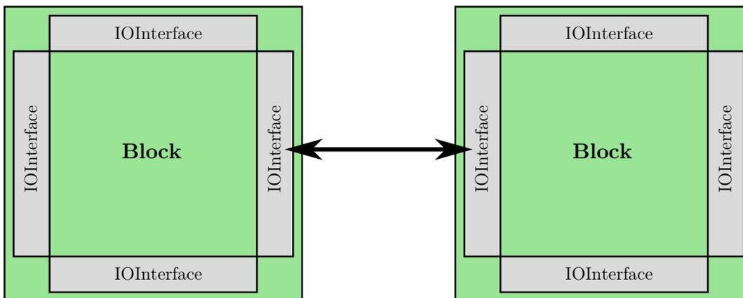
Figure 3-10 – **Block model used in the *vbsgen* framework.** *Each element of the model array derives from the root type *Block* of the *vbsgen* framework. A *Block* contains *IOInterface*s on all of its four sides. These interfaces model the connection points between the block and its neighbors and serve to determine the relationships between elements of the model array during the bit-stream generation.*
