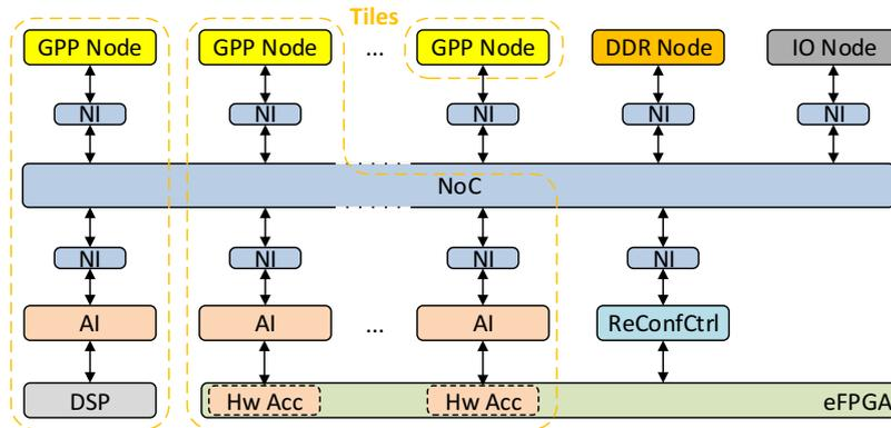
Figure 7-2 – Overview of the FlexTiles platform heterogeneous many-core hardware architecture [Jan+15].
