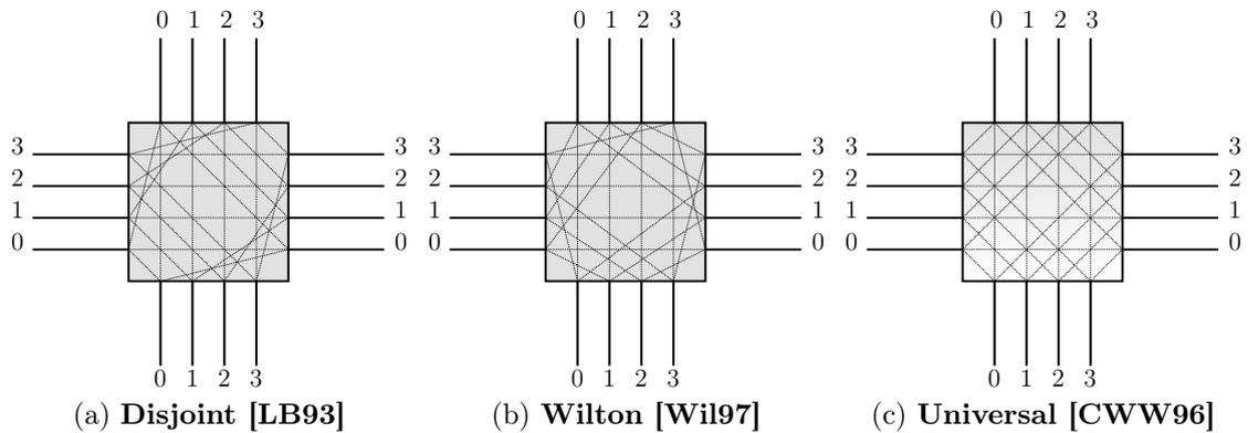
Figure 1-14 – **Switch block topologies.** Various switch block topologies have been explored, the disjoint, Wilton and universal models are three possible switch block implementations. While the disjoint topology may simplify the global-to-detailed routing step of the CAD flow, the Wilton topology shows an increased flexibility which can lead to fewer tracks used. The universal model meets the dimensional constraint but fails to be easily expendable to segmented routing schemes.
