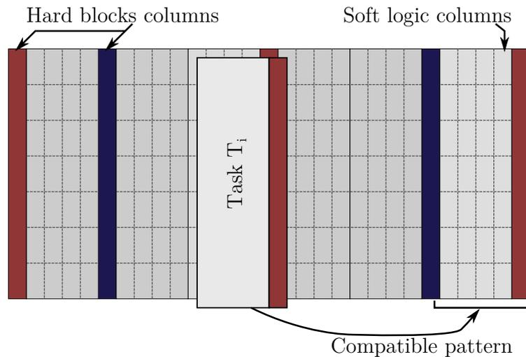
Figure 2-1 – **Compatible patterns on a logic fabric for task relocation.** *The geometry of task  $T_i$  as well as the order of soft logic and hard block columns composing it must be preserved to allow for its relocation. Considering these constraints, the technique in [Kra+06] can only relocate  $T_i$  to the rightmost position.*
