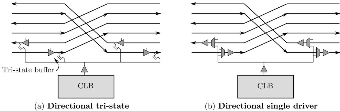
Figure 1-16 – **Directional tristate and single driver implementations of unidirectional output drivers [Lem+04].** *Directional routing can be implemented in an architecture using pass-transistors and tri-state buffers for each logic block input or output. Another single driver implementation may be considered, which complicates the architecture design but cancels the need for tri-state buffers.*
