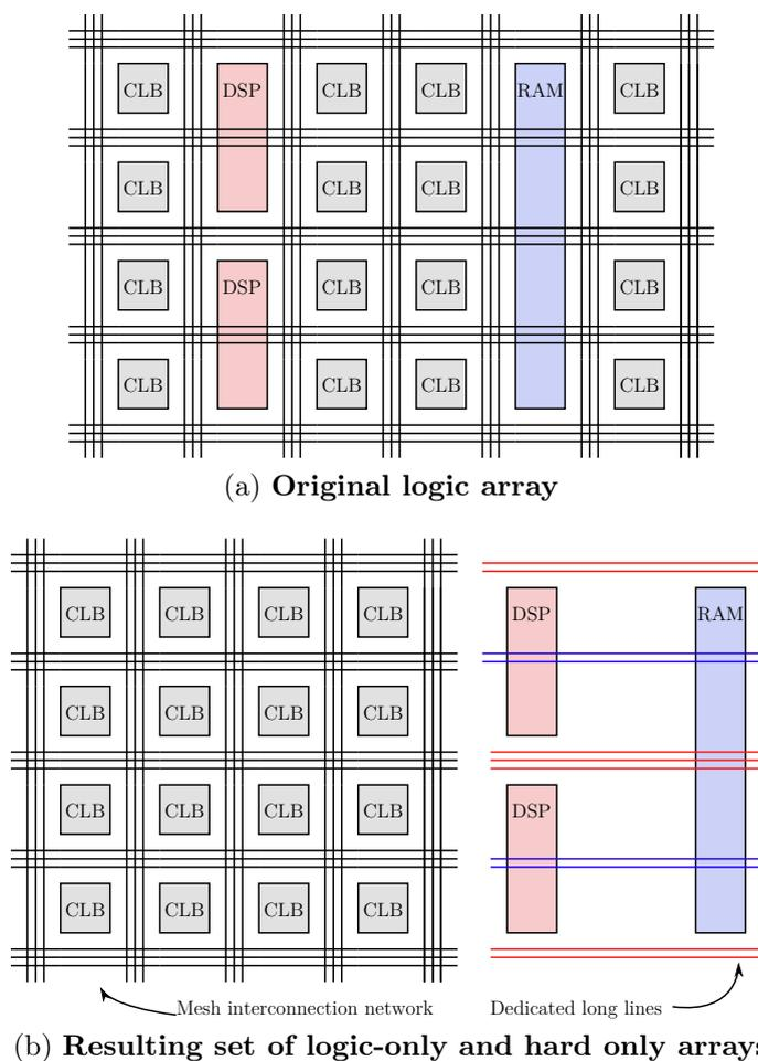
Figure 5-2 – **Abstraction of heterogeneous resources.** *The original logic array, based on an island-style architecture, contains CLBs as soft logic elements and two types of hard blocks. The interconnection network is shared by both soft and hard blocks. In the abstraction of the logic array, the soft logic lies in one mesh interconnect network dissociated from the hard block routing. The connection to and from hard blocks is made via long lines dedicated to each type of hard block.*
