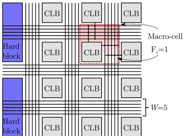
Figure 3-2 – **Example of an island-style architecture and its repeatable macro-cell.** The considered architecture is a generalized island-style logic array and its mesh routing network. Ignoring localized heterogeneity, a repeatable pattern can be identified, duplicated in both directions, which is what we consider in this document as a macro-cell.
