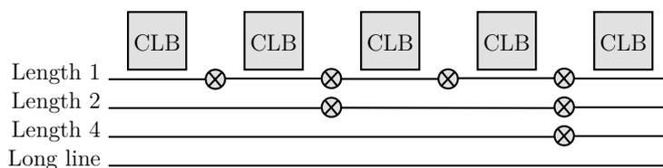
Figure 1-11 – **Example of a distribution of routing tracks in an interconnect architecture.** *A wide distribution of the segment length over the device allows longer path to use less routing resources. The decreased wire capacitance has a direct impact on the wire delay which is substantially lower than with multiple smaller segments.*
