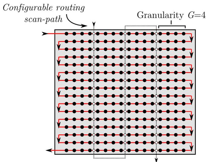
Figure 6-8 – **A configurable shift-register.** *The configurable shift-register uses the routing element capabilities to shortcut or forward the configuration signal. The routing elements are spaced by  $G$  frames to allow for a fine or gross placement, tasks must however be sized accordingly. The configurable routing elements are effectively chained together in a second scan-path which needs to be programmed prior to the insertion of the task data.*
