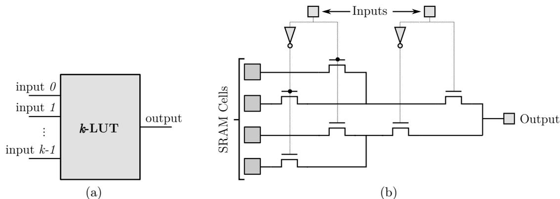
Figure 1-4 – **Architecture of a 2-LUT using memory cells and pass-transistors.** In an SRAM FPGA device, the most convenient way of implementing multiplexers is to use pass-transistors. The implementation of a  $k$ -LUT requires  $2^k$  memory cells and a  $k$ -to-1 multiplexer, here implemented using a tree of pass-transistors, although more optimized versions are more commonly used.
