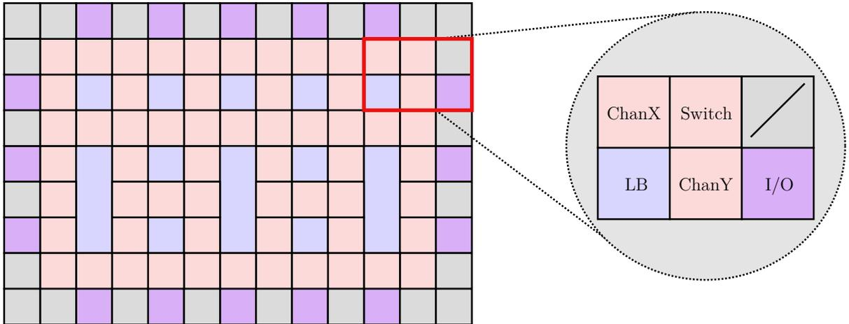
Figure 3-9 – **The *vbsgen* model array.** *The internal model of an architecture in vbsgen is a two dimensional array where each element represents one basic feature of the FPGA: soft logic, routing, input/outputs, etc. Each block relies on a specialization of classes of the model framework. Once built, the model array is populated using placement and routing data, and eventually dumped as a bit-stream.*
