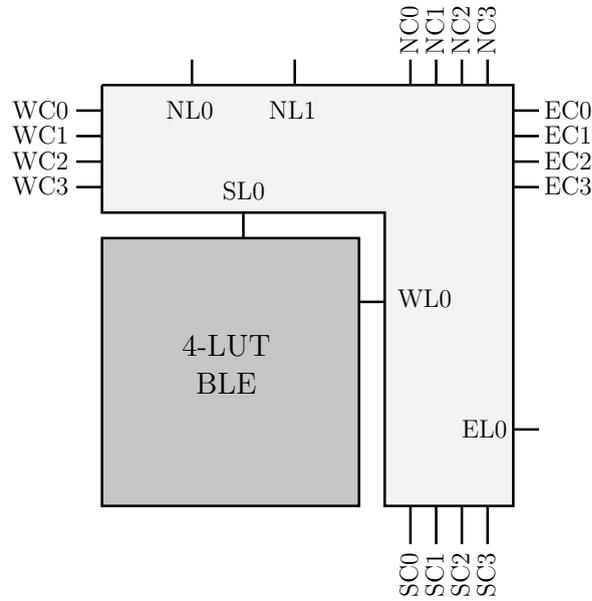
Figure 4-2 – **Example macro-cell architecture with  $W = 4$  and  $L = 5$ .**
