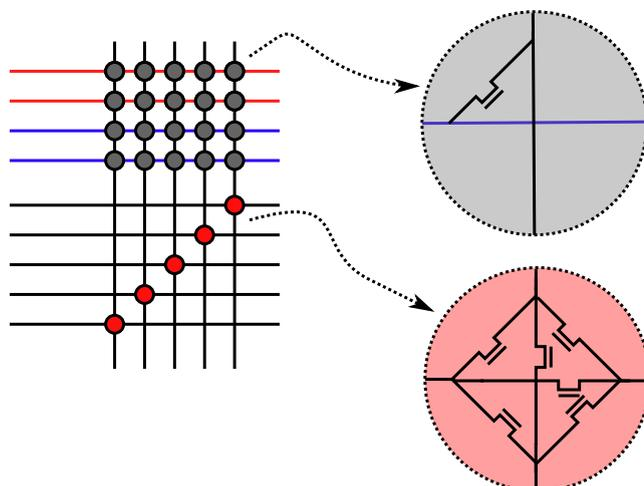
Figure 5-3 – **Switch box enhanced to include connections between heterogeneous and homogeneous layers.** *The red and blue horizontal wires (the top four wires) represent heterogeneous-only long lines while the remaining black wires represent homogeneous routing. The interconnection between the heterogeneous-only long lines and the homogeneous routing is made through connection points at the switch level.*
