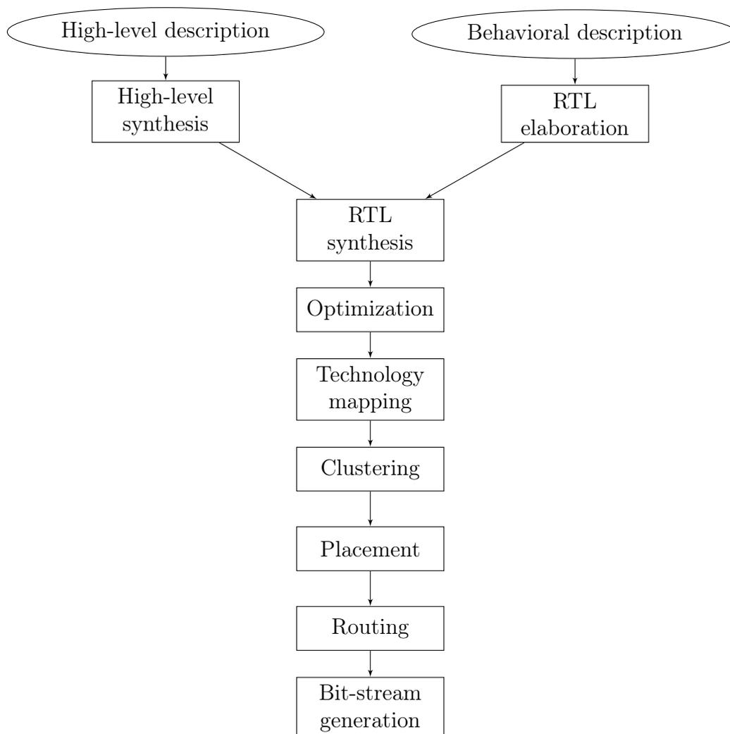
Figure 2-3 – A typical FPGA design flow
