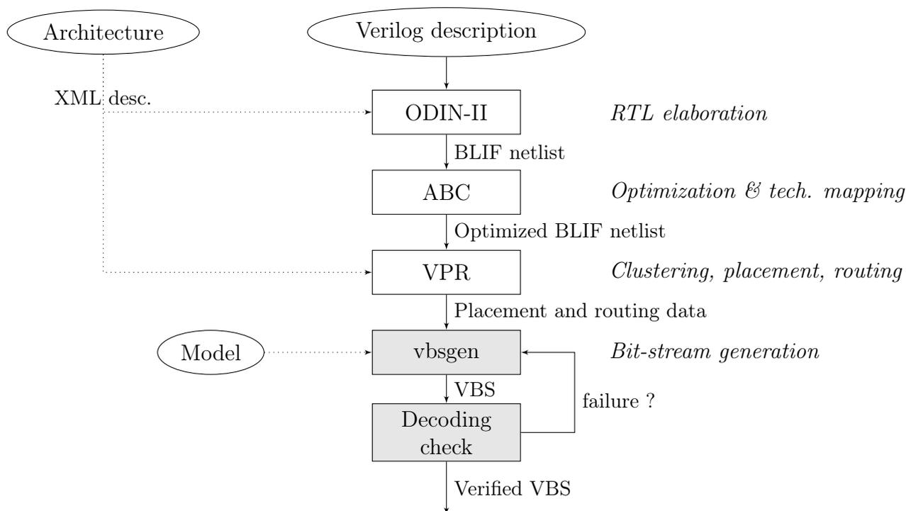
Figure 3-7 – **The Virtual Bit-Stream design flow, based on the Verilog-To-Routing framework.** *The Virtual Bit-Stream design flow relies on the Verilog-To-Routing framework to generate placement and routing data. The vbsgen back-end is subsequently used to generate custom bit-streams using a custom model. A decoding step is added after the bit-stream generation to ensure that the Virtual Bit-Streams created will be decodable at runtime, and to regenerate non-compliant bit-streams.*
