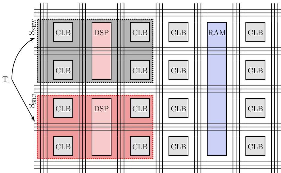
Figure 5-1 – **Relocation problem in modern FPGAs.** Task  $T_1$ , placed on a set  $S_{src}$  of resources, is only movable to another set  $S_{new}$  with resource types and positions matching those in the original set. The necessity to find matching partitions to perform the relocation of a task hampers the overall placement flexibility of the device.
