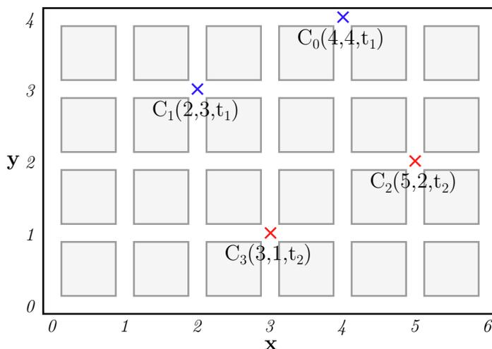
Figure 5-5 – **Model of a task with abstracted heterogeneous hard blocks.** Tasks are defined as a set of homogeneous logic elements and a variable number of connections  $C_i$  to hard blocks. Each connection  $C_i$  has to be linked to a hard block via heterogeneous-only routing. A valid placement of a task needs to satisfy the connection type constraint for all the connections.
