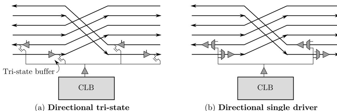
Figure 7-6 – **Uni-directional routing in modern architectures.**
