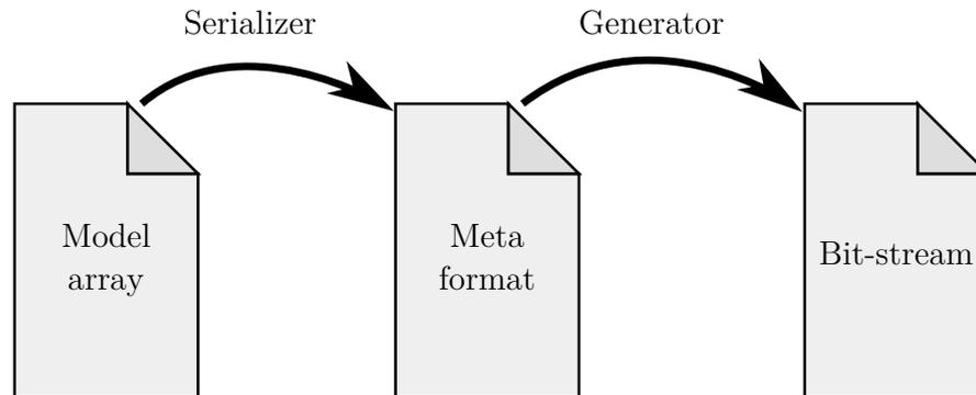
Figure 3-11 – **Generation of intermediate representations and final bit-stream in the *vbsgen* framework.** *From the designer perspective, the user-supplied vbsgen model fills a meta-structure dedicated to a specific output format (e.g. virtual or conventional bit-stream) instead of actually creating binary structures, using a user-defined Serializer. The conversion process from the meta-structure to the final bit-stream is ensured by a Generator included in the framework.*
