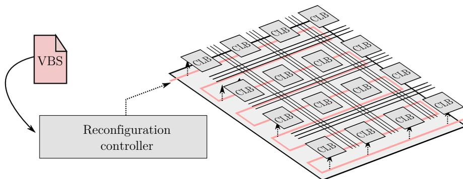
Figure 3-1 – **Overview of the Virtual Bit-Stream technique integrated to a FPGA logic fabric.** *The Virtual Bit-Streams are decoded by a dedicated reconfiguration controller which decodes the alternate representation and loads it into the target logic fabric configuration memory.*
