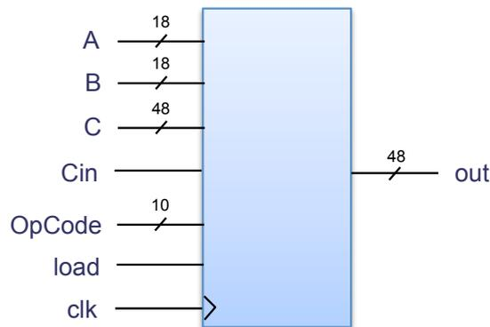
Figure A-6 – Arithmetic accelerator (DSP block) overview
