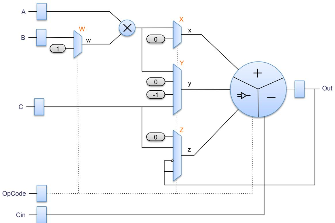
Figure A-7 – Details of an arithmetic accelerator
