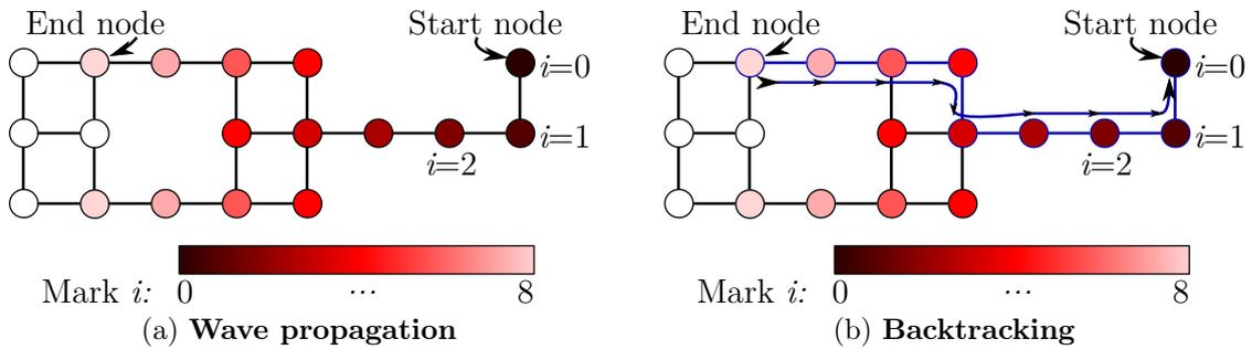
Figure 2-4 – **Illustration of the maze routing algorithm.** The first step incrementally marks neighboring nodes with an increasing  $i$  mark from the start node, until the end node gets marked. The second step builds the final path starting from the end node by backtracking decreasing marks. The maze algorithm ensures that the shortest possible path is built, although multiple of them are possible for a given routing graph.
