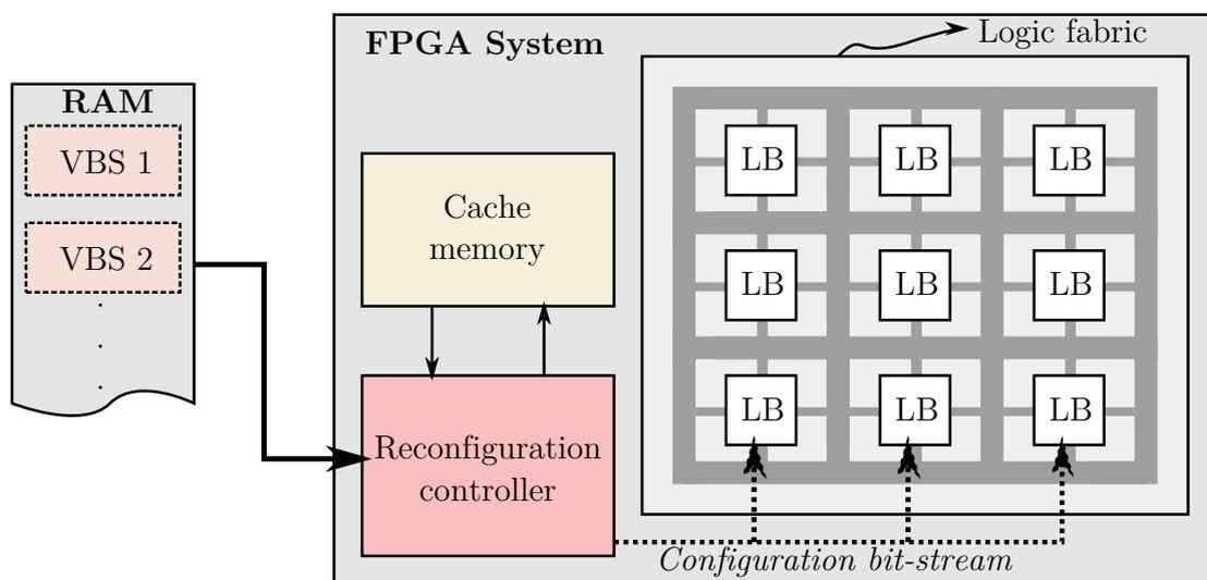
Figure 3-12 – **Integration of the Virtual Bit-Stream technique in an FPGA system.** *The support of Virtual Bit-Stream loading at runtime in a FPGA system is brought by an online controller realizing the online decoding of the Virtual Bit-Stream files in real time. The controller integrates a decoding pipeline allowing to read, decode and create a conventional bit-stream on the fly from the Virtual Bit-Stream for a given location in the logic fabric.*
