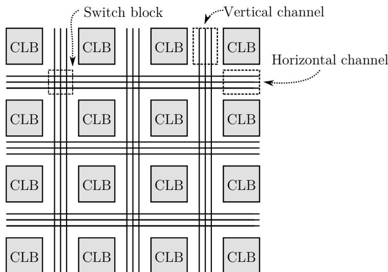
Figure 1-13 – **Overview of an island-style interconnect architecture.** *Island-style architectures have regular logic fabric and routing interconnect. The routing network is split in vertical and horizontal channels. Switch blocks allow interconnecting the channels at their intersections.*
