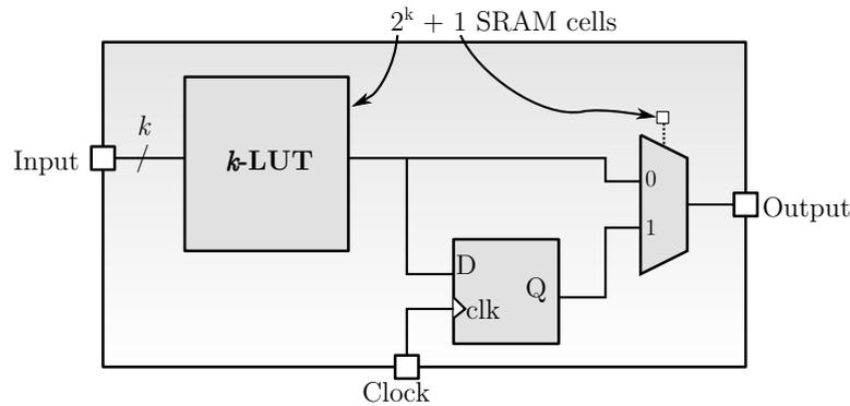
Figure 1-5 – **Overview of a basic logic block.** *The basic logic block comprises a  $k$ -LUT to provide the logic flexibility, associated with a D flip flop to synchronize the LUT output with the clock. A multiplexer on the output path enables the selection of the asynchronous or synchronous LUT output to allow for complex logic chains.*
