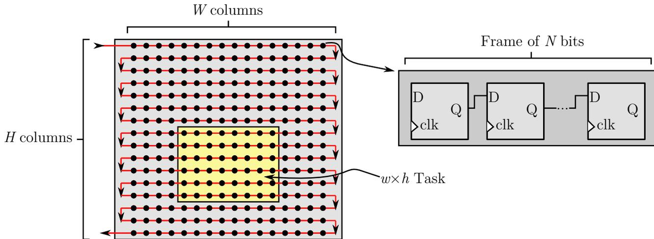
Figure 6-6 – **Basic organization of a standard of hybrid scan-path over the programmable device.** *The static scan-path traverses the configuration memory in a serpentine way, line by line. The considered smallest units of configuration are frames of  $N$  configuration bits.*
