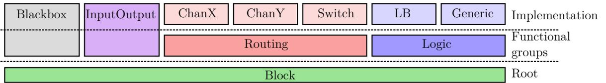
Figure 3-8 – **The *vbsgen* model framework.** *The framework is a collection of pre-defined blocks that may be directly used in a new architecture model. The root type `Block` is split in four functional groups, themselves split in more specific blocks. The framework includes the main soft logic and routing resources and their interconnection capabilities.*
