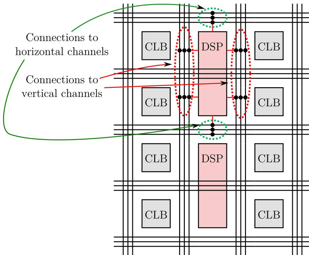
Figure 5-7 – **Limitations of the enhanced architecture in VPR.** *The VPR internal model allows connections from a hardware block to vertical routing channels on every side of all the grid positions occupied by the block. On the other hand, connections to horizontal routing channels are only made on the top and bottom sides of the block, leading to congestions of the routing signals on a few channels with the enhanced routing model.*
