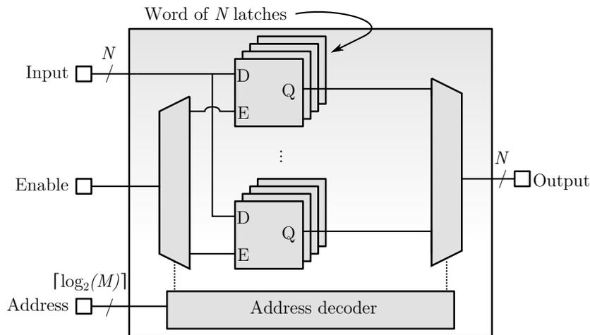
Figure 6-1 – **An array of memory cells accessible with word addressing.** *The word-addressing scheme allows to directly target one of the word of the memory. Single bits however needs to be accessed as part of their word. A combinatorial address decoder is responsible for the generation of the enable signal when the latches are written, and of the output selection when the latches are read.*
