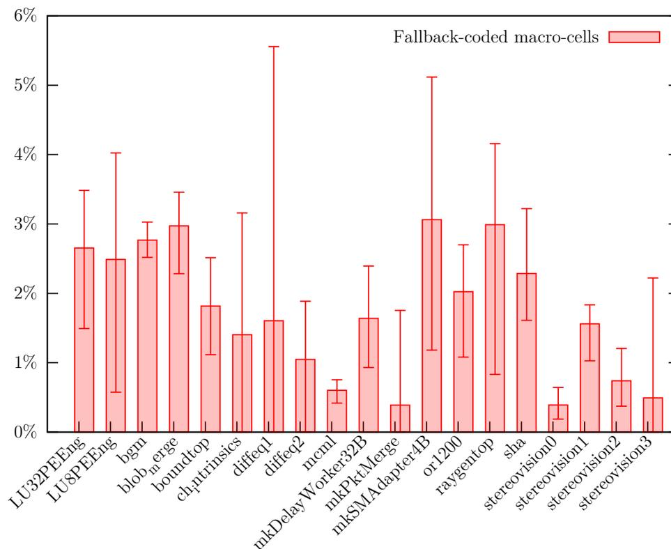
Figure 4-7 – **Normalized number of fallback-coded macro-cells with the LUT algorithm for each design of the VTR benchmark set.** *The average percentage of fallback-coded macro-cells indicates how many times the algorithm fails over the set of macro-cells of each design. The error bars represent the maximum and minimum values of the percentage of fallback-coded macro-cells over the 10 different place and route trials of the benchmark set.*
