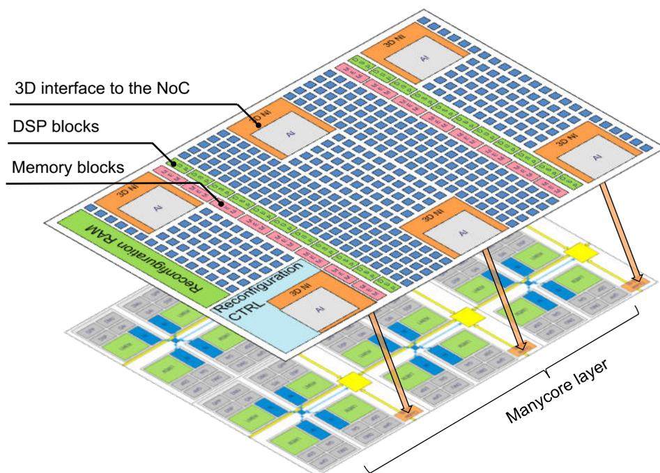
Figure 7-1 – **The 3-D stacked FlexTiles platform.** *The FlexTiles platform is a 3-D stacked heterogeneous architecture comprising GPP, DSP and hardware tasks loaded onto an embedded FPGA (eFPGA). The communication between these elements is made through a NoC. Communications between the eFPGA and the manycore layer is realized with 3-D links to the NoC with dedicated interfaces in the FPGA logic fabric.*
