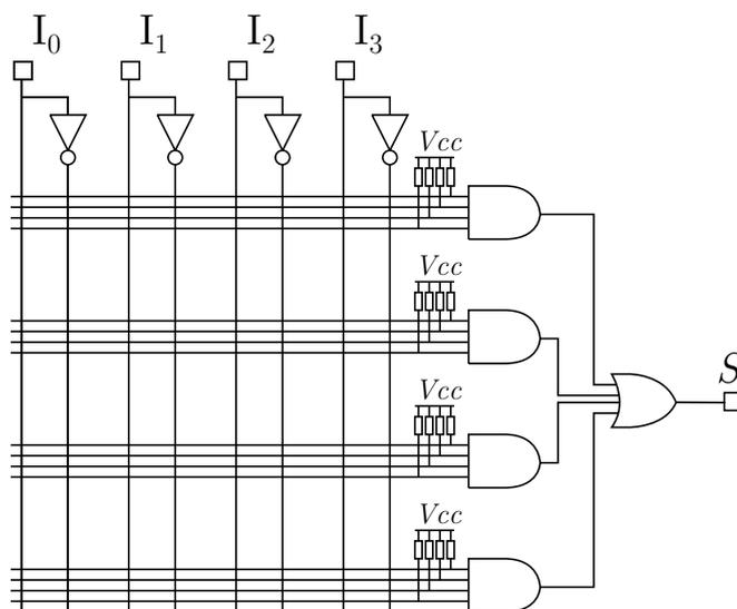
Figure 1-1 – **Details of the configurable sum-of-products in a PAL.** *The four inputs  $I_{0..3}$  and their inverse are tied to a crossbar interconnect with the AND-gate inputs. In PALs, the AND outputs are OR-ed together to form the output, but subsequent technologies such as Programmable Logic Arrays (PLAs) added another crossbar to yield multiple outputs.*
