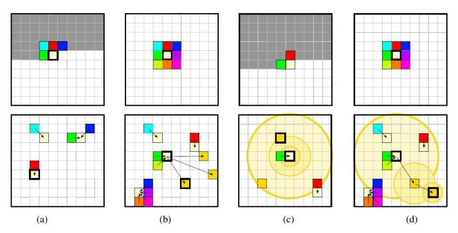
**Figure 3.7:** (a) Coherent candidates. (b) *k*-coherent candidates. (c) Search performed by PatchMatch: A random search is carried around each coherent candidate with decreasing radius. (d) Random search strategy of Busto et al. : A random walk is performed with decreasing radius. The walk steps if an improving candidate is found. Figure from Busto et al.
