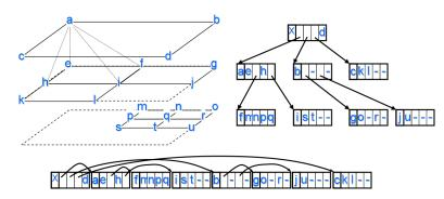
Figure 4.11: Example of a primal autumnal tree and its memory packing. Dashes denote undefined data values.
