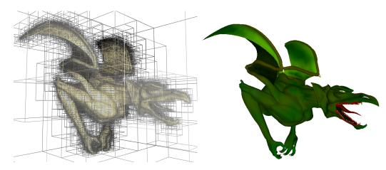
**Figure 4.2:** Left: The 3D hierarchy. Each node is regularly subdivided in  $2^3$  nodes (octree). Each internal node stores the average color of the children. Leaf nodes are painted by the artist. Right: Rendering using the texture stored in the octree.
