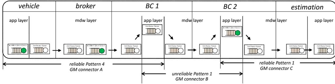
Figure 5.14: End-to-end queuing network for the `vehicle-device`  $\rightarrow$  `estimation-service` interconnection.
