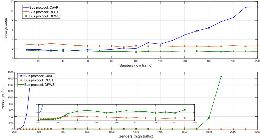
Figure 3.19: Response times for one-way interactions through REST, CoAP and DPWS bus protocols in scenarios 1, 2 and 3.
