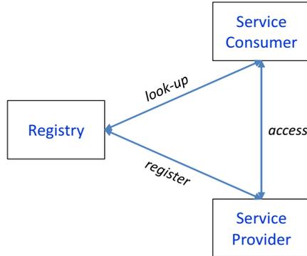
Figure 2.2: Service-oriented architecture (SOA).
