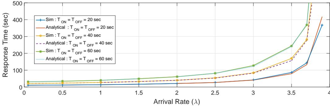
Figure 5.16: Analytical vs. simulated response times at the ON/OFF queueing center.
