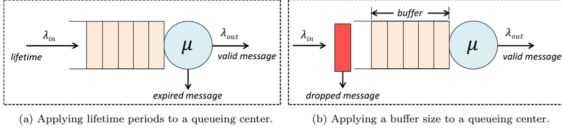
Figure 5.4: Queues with message expirations and finite capacity.
