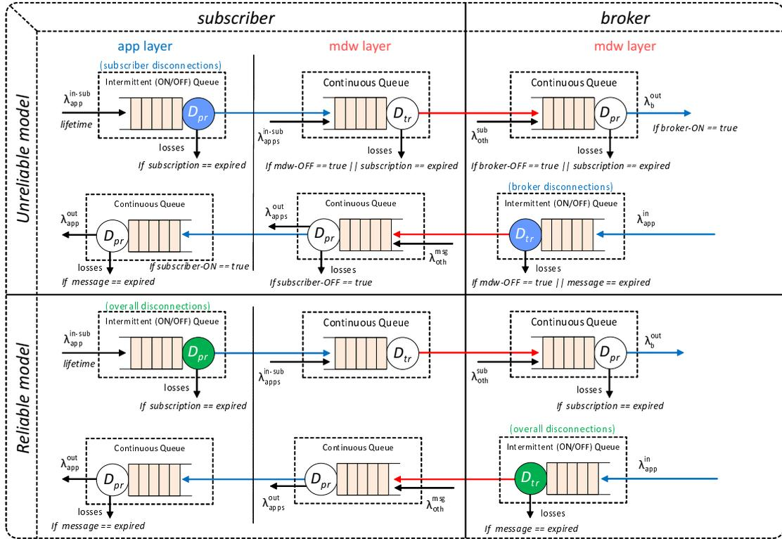
Figure 5.11: PerfMP for PS two-way stream interactions.
