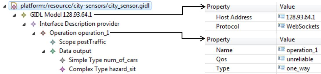
Figure B.3: GIDL model for fixed-sensors.
