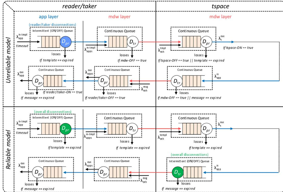
Figure 5.13: PerfMP for TS two-way sync interactions.
