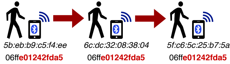
Figure III.1 – Representation of a successful attack. The BLE device is randomizing its BD_ADDR (in italic ) over time while keeping a static identifier (in bold ) in the advertising data. Such a 5-byte identifier can be used by a passive attacker to link together the packets generated with the three different BD_ADDR.
