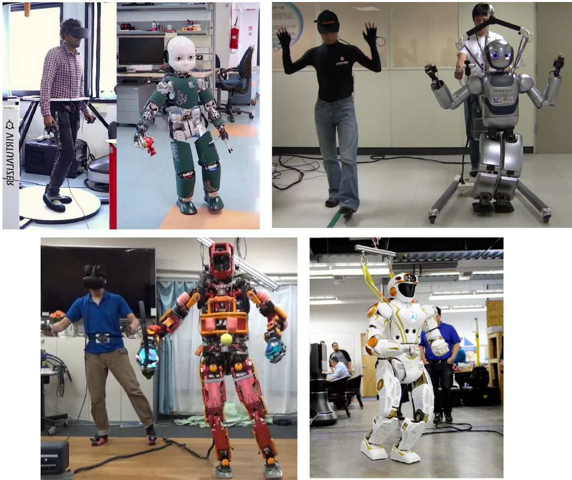
Figure 4.1: Examples of teleoperated locomotion. Top-left: iCub robot teleoperated with a VR walking platform [55]; top-right: walking imitation of MAHRU robot [97]; bottom-left: whole-body teleoperation of a stepping motion with the robot JAXON [79]; bottom-right: remote guidance of the walking of the Valkyrie robot through a GUI [87].
