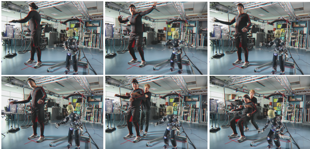
Figure 2.10: Snapshots from the teleoperation experiment. The robot does not fall when the human operator falls back (frame on the bottom-right).
